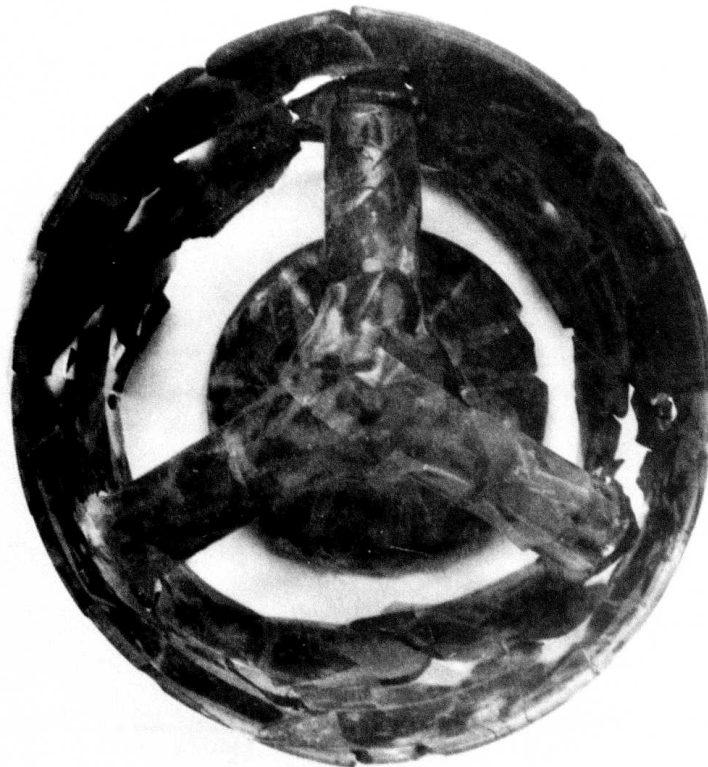
Figure 3.18 — Reconstructed Nose Cone after Failure of Rotor 1195
